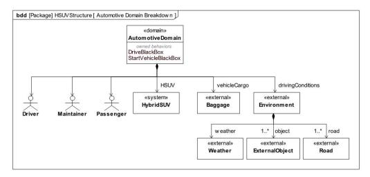
Figure D.15 Defining the Automotive Domain (compare with Figure D.4) – (Block Definition Diagram)
