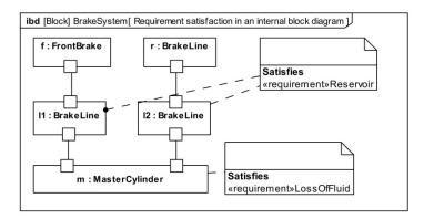
Figure 16-4: Requirement satisfaction in an internal block diagram
