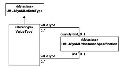
Figure 8-4: Abstract syntax extensions for SysML value types
