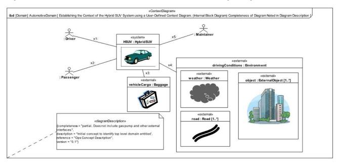
Figure D.4 Establishing the Context of the Hybrid SUV System using a User-Defined Context Diagram. (Internal Block Diagram) Completeness of Diagram Noted in Diagram Description
