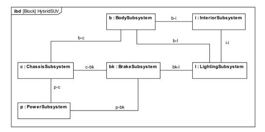
Figure D.17 Internal Structure of Hybrid SUV (Internal Block Diagram)
