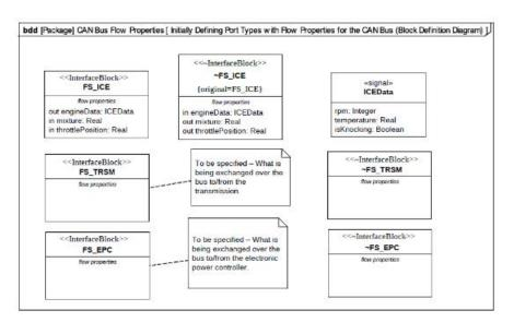
Figure D.21 Initially Defining Port Types with Flow Properties for the CAN Bus (Block Definition Diagram)
