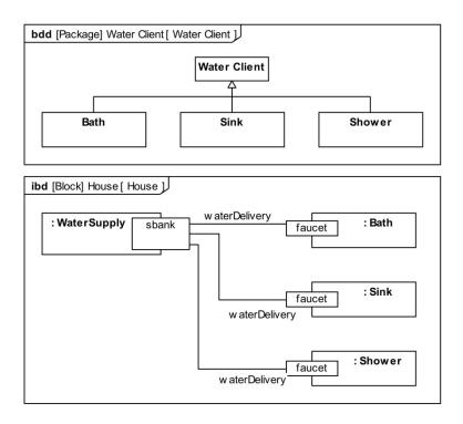
Figure 9-11: Specializations of Water Client in house example
