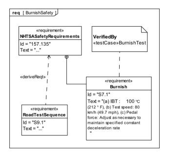
Figure 16-6: Linkage of a Test Case to a requirement: This figure shows the Requirement Diagram
