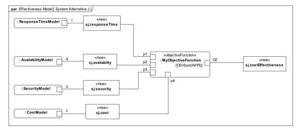
Figure E.4 Example Parametric Diagram using Stereotypes for Measures of Effectiveness
