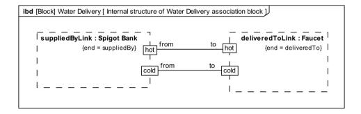
Figure 9-9: Internal structure of Water Delivery association block
