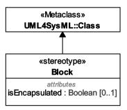
Figure 8-2: Abstract syntax extensions for SysML blocks
