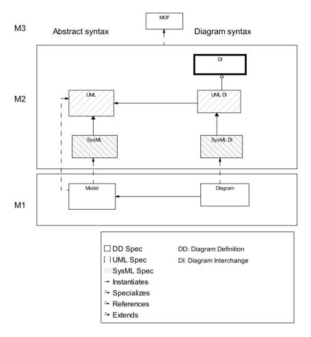
Figure B.1: SysML DI architecture
