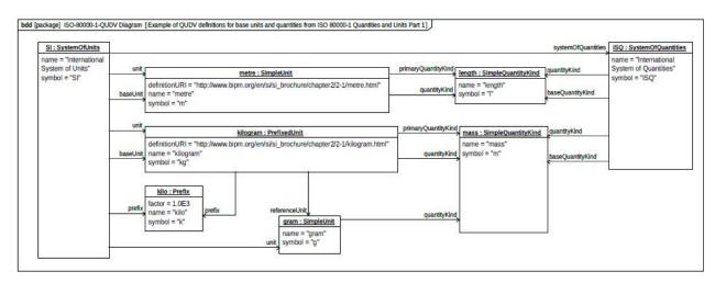
Figure E.8 Base Unit and Quantity Kinds of the SI and ISQ respectively
