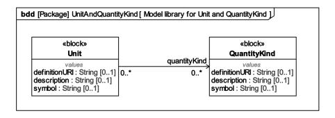
Figure 8-11: Model library for Unit and QuantityKind
