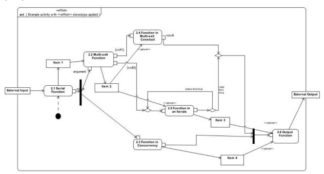
Figure E.1 Example activity with «effbd» stereotype applied
