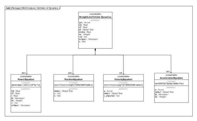
Figure D.34 Defining Straight-Line Vehicle Dynamics Mathematical Constraints (Block Definition Diagram)
