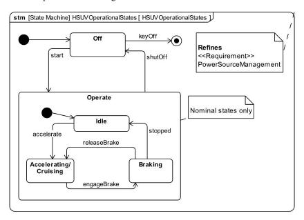
Figure D.8 Finite State Machine Associated with "Drive the Vehicle" (State Machine Diagram)
