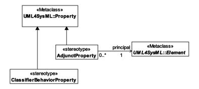
Figure 8-9: Abstract syntax extensions for SysML adjunct properties and classifier behavior properties
