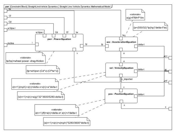
Figure D.33 Straight Line Vehicle Dynamics Mathematical Model (Parametric Diagram)
