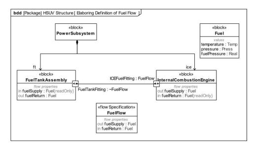
Figure D.23 Elaborating Definition of Fuel Flow. (Block Definition Diagram)
