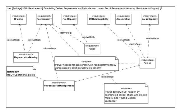
Figure D.12 Establishing Derived Requirements and Rationale from Lowest Tier of Requirements Hierarchy (Requirements Diagram)
