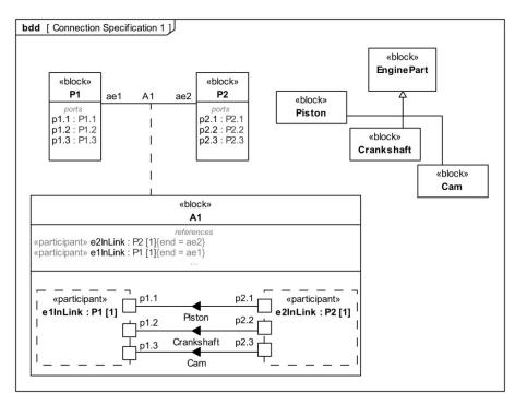
Figure 9-16: Usage example of item flow decomposition
