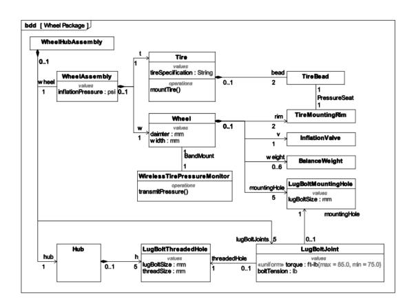
Figure 8-12: Block diagram for the Wheel Package
