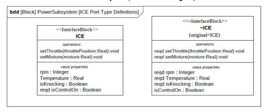
Figure D.20 Blocks Typing Ports in the Power Subsystem (Block Definition Diagram)
