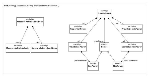
Figure D.37 Decomposition of "Accelerate" Function (Block Definitions diagram)
