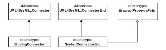
Figure 8-6: Abstract syntax extensions for SysML connector ends
