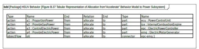
Figure D.40 Tabular Representation of Allocation from "Accelerate" Behavior Model to Power Subsystem (Table)
