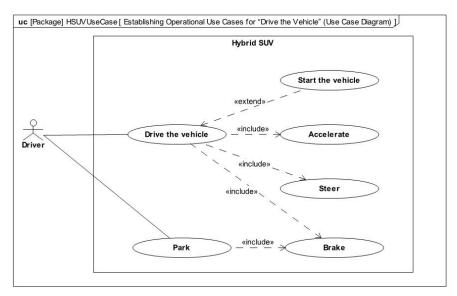
Figure D.6 Establishing Operational Use Cases for "Drive the Vehicle" (Use Case Diagram)
