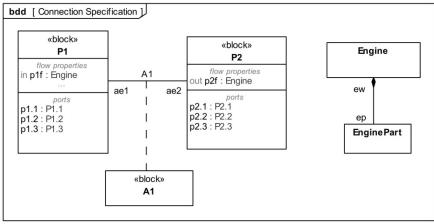
Figure 9-17: Usage example of item flow decomposition
