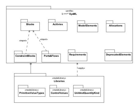
Figure 4-3: SysML Package Structure
