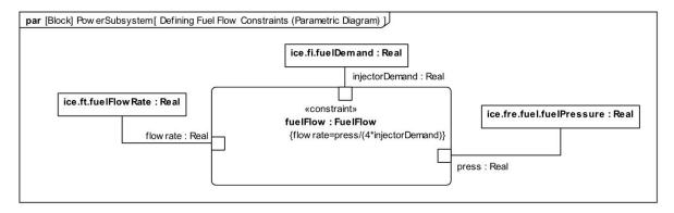
Figure D.24 Defining Fuel Flow Constraints (Parametric Diagram)
