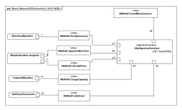
Figure D.31 Defining Measures of Effectiveness and Key Relationships (Parametric Diagram)
