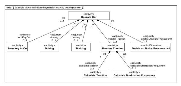
Figure 11-13: Example block definition diagram for activity decomposition
