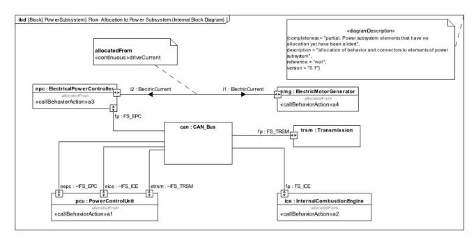
Figure D.39 Flow Allocation to Power Subsystem (Internal Block Diagram)
