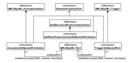
Figure 9-2: Stereotypes for Actions on Nested Ports
