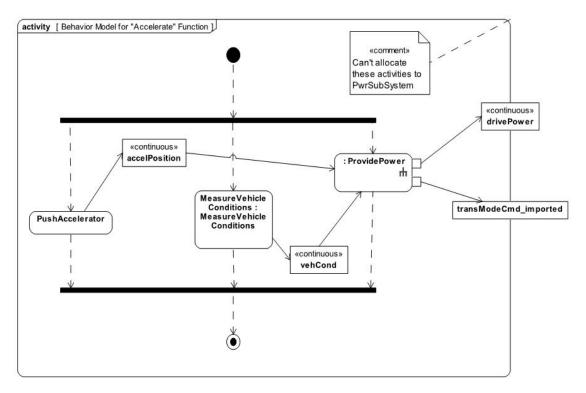
Figure D.36 Behavior Model for "Accelerate" Function (Activity Diagram)
