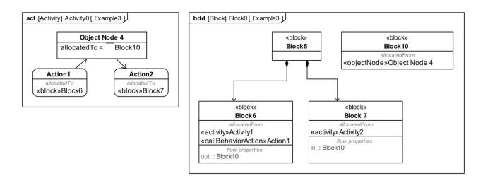
Figure 15-7: Example of flow allocation from ObjectNode to FlowProperty
