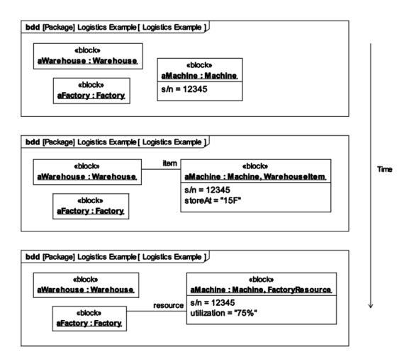
Figure 8-23: Changes in classification over time due to property-specific types
