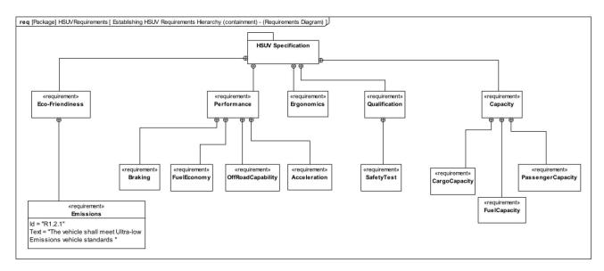
Figure D.11 Establishing HSUV Requirements Hierarchy (containment) - (Requirements Diagram)
