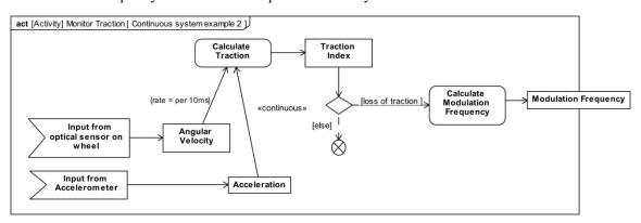
Figure 11-11: Continuous system example 2
