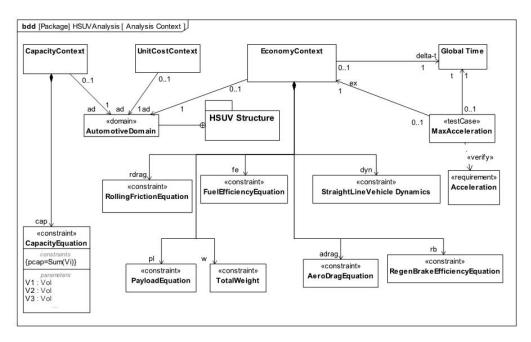
Figure D.26 Defining Analyses for Hybrid SUV Engineering Development (Block Definition Diagram)
