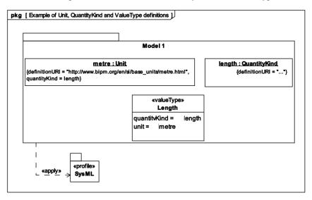
Figure 8-18: Example of Unit, QuantityKind and ValueType definitions
