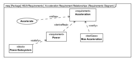
Figure D.13 Acceleration Requirement Relationships (Requirements Diagram)
