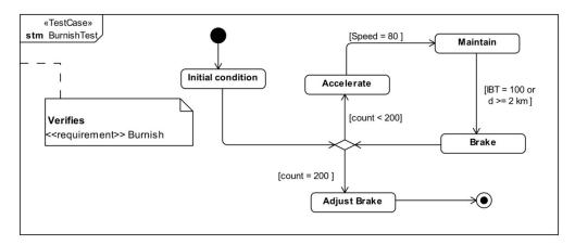
Figure 16-7: Linkage of a Test Case to a requirement: This figure shows the Test Case as a State Diagram
