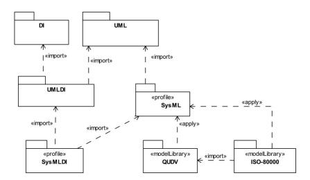
Figure 4-4: Non-normative Package Structure
