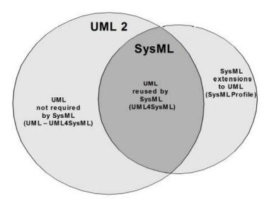
Figure 4-1: Overview of SysML/UML Interrelationship
