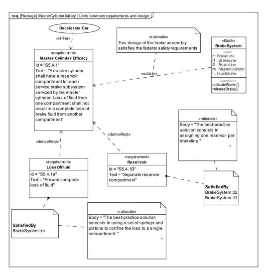
Figure 16-3: Links between requirements and design
