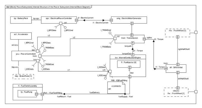
Figure D.19 Internal Structure of the Power Subsystem (Internal Block Diagram)
