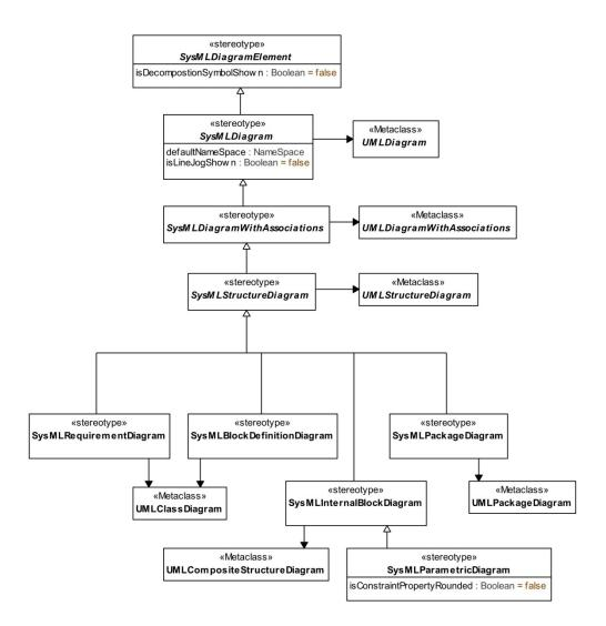
Figure B.3: Abstract syntax extensions for SysML diagrams (1)
