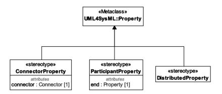
Figure 8-3: Abstract syntax extensions for SysML properties
