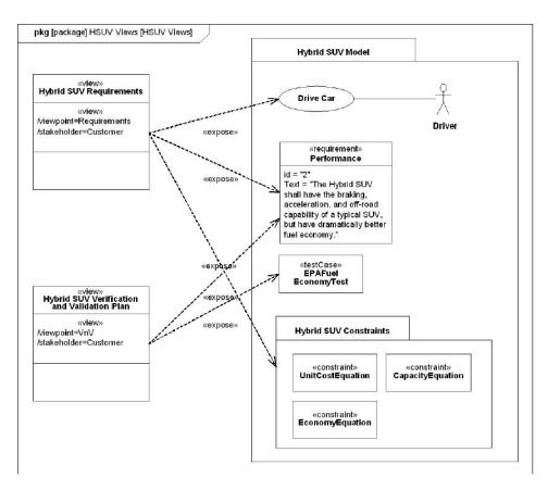
Figure D.29 Requirements and VnV views exposing elements from the model (Package Diagram)
