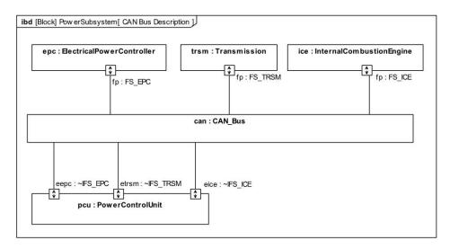
Figure D.22 Consolidating Connectors into the CAN Bus. (Internal Block Diagram)
