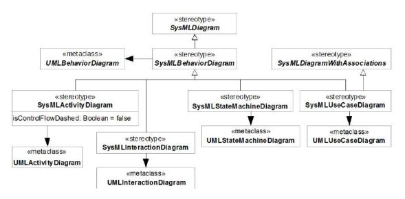
Figure B.4: Abstract syntax extensions for SysML diagrams (2)
