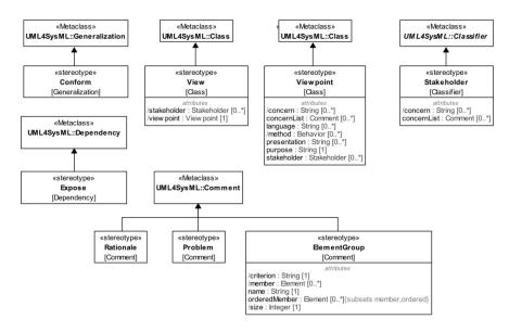
Figure 7-1: Stereotypes defined in package ModelElements
