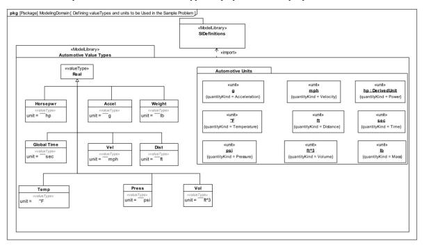
Figure D.2: Defining value Types and units to be used in the Sample Problem
