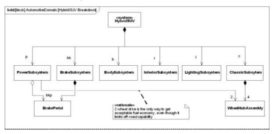
Figure D.16 Defining Structure of the Hybrid SUV System (Block Definition Diagram)
