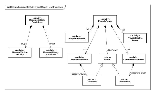
Figure C.34 - Decomposition of "Accelerate" Function (Block Definition diagram)
