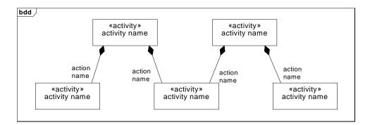
Figure 11.1 - Block definition diagram with activities as blocks
