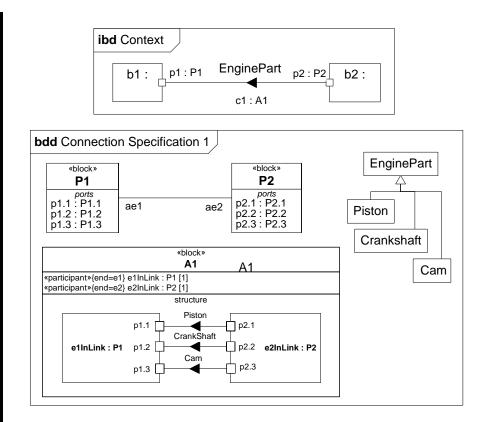
Figure 9.16 - Usage example of item flow decomposition
