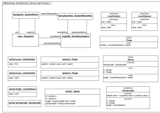
Figure D.13 - Spring Length Example
