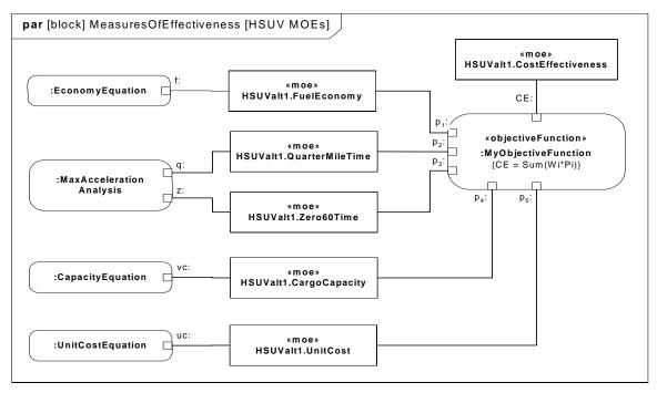
Figure C.28 - Defining Measures of Effectiveness and Key Relationships (Parametric Diagram)
