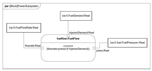
Figure C.24 - Defining Fuel Flow Constraints (Parametric Diagram)
