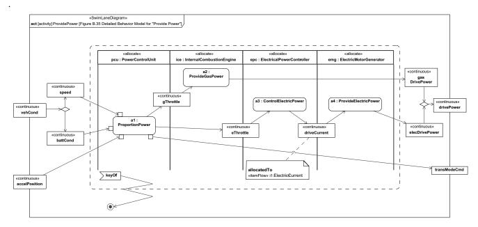
Figure C.35 - Detailed Behavior Model for "Provide Power" (Activity Diagram) Note hierarchical consistency with Figure C.33.
