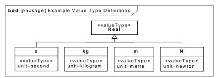
Figure 8.10 - Defining Value Types with units of measure from the International System of Units (SI)
