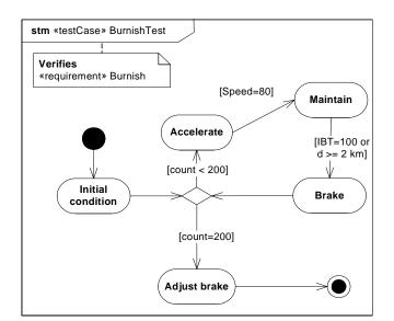
Figure 16.8 - Linkage of a Test Case to a requirement: This figure shows the Test Case as a State Diagram
