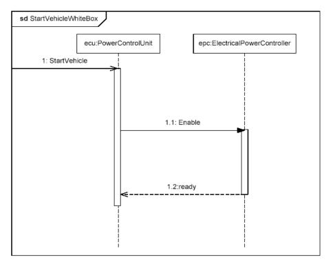
Figure C.10 - White Box Interaction for "StartVehicle" (Sequence Diagram)
