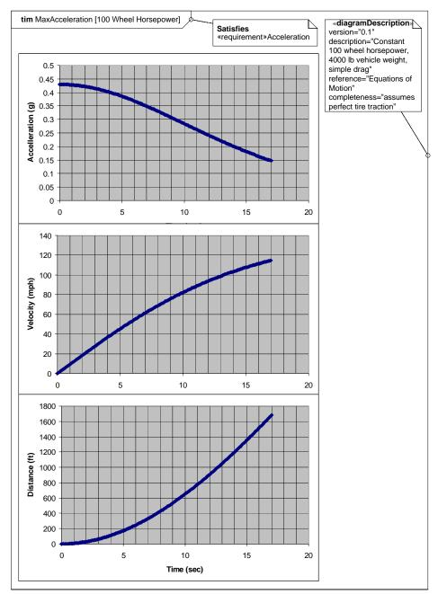
Figure C.32 - Results of Maximum Acceleration Analysis (Timing Diagram)
