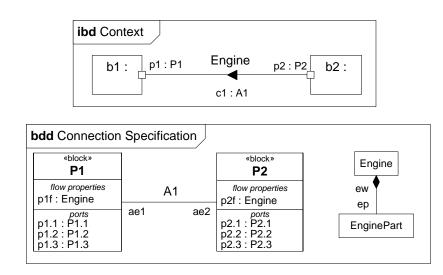
Figure 9.17 - Usage example of item flow decomposition
