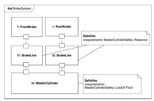
Figure 16.5 - Requirement satisfaction in an internal block diagram.
