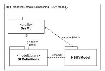
Figure C.1 - Establishing the User Model by Importing and Applying SysML Profile & Model Library (Package Diagram)
