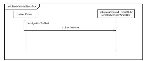
Figure C.9 - Black Box Interaction for "StartVehicle," referencing White Box Interaction (Sequence Diagram)
