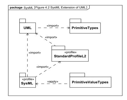
Figure 4.2 - SysML Extension of UML
