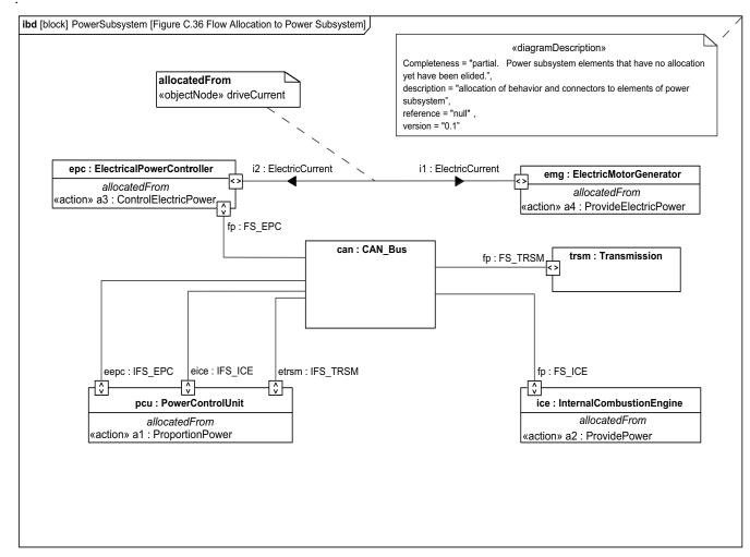
Figure C.36 - Flow Allocation to Power Subsystem (Internal Block Diagram)
