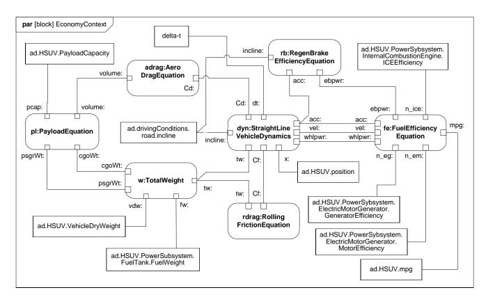
Figure C.29 - Establishing Mathematical Relationships for Fuel Economy Calculations (Parametric Diagram)
