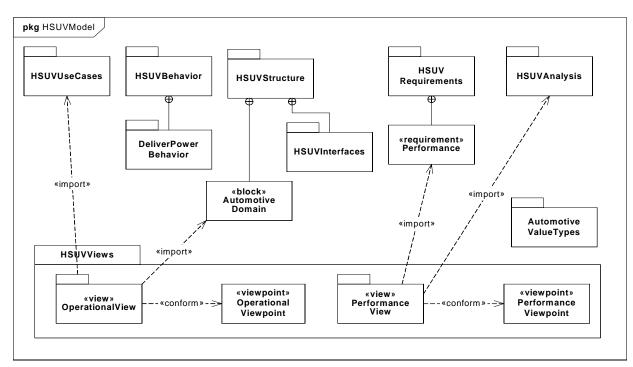
Figure C.3 - Establishing Structure of the User Model using Packages and Views (Package Diagram)
