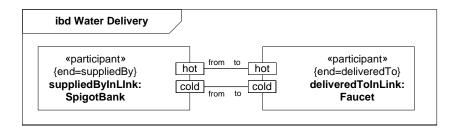
Figure 9.9 - Internal structure of Water Delivery association block
