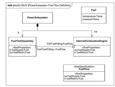
Figure C.23 - Elaborating Definition of Fuel Flow. (Block Definition Diagram)
