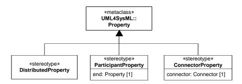
Figure 8.3 - Abstract syntax extensions for SysML properties
