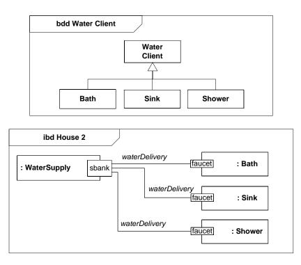
Figure 9.11 - Specializations of Water Client in house example
