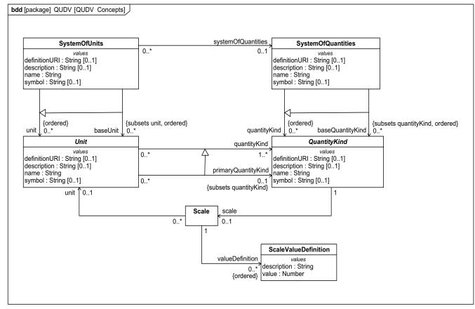
Figure D.8 - QUDV Concepts diagram
