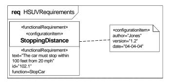
Figure 17.9 - Using two stereotypes on a model element
