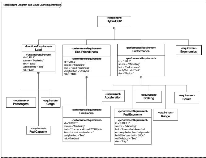
Figure D.3 - Example extensions to Requirement
