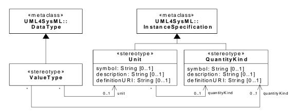
Figure 8.4 - Abstract syntax extensions for SysML value types
