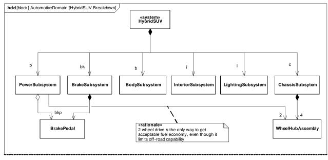
Figure C.16 - Defining Structure of the Hybrid SUV System (Block Definition Diagram)
