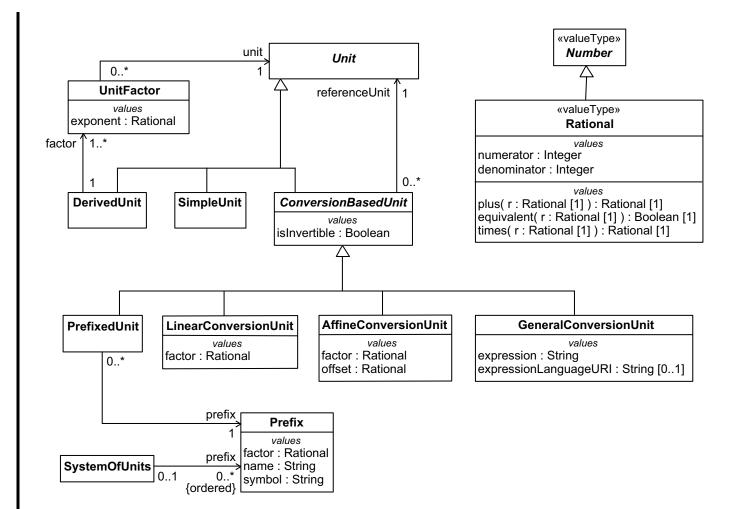
Figure D.9 - QUDV Units diagram
