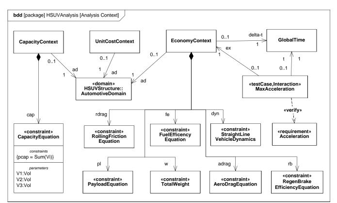
Figure C.26 - Defining Analyses for Hybrid SUV Engineering Development (Block Definition Diagram)
