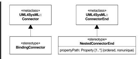
Figure 8.5 - Abstract syntax extensions for SysML connector ends
