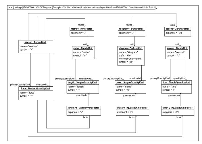
Figure D.12 - Example of a derived unit and derived quantity kind
