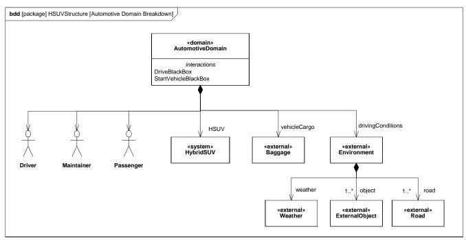
Figure C.15 - Defining the Automotive Domain (compare with Figure C.4) - (Block Definition Diagram)
