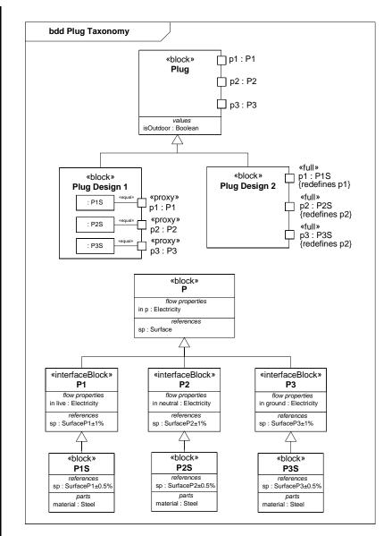
Figure 9.7 Usage example of proxy and full ports
