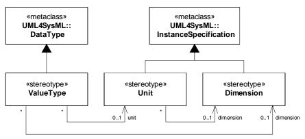
Figure 8.4 - Abstract syntax extensions for SysML value types
