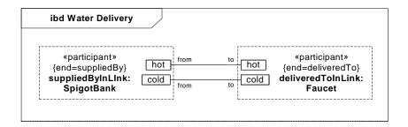
Figure 8.13 - Internal structure of Water Delivery association block
