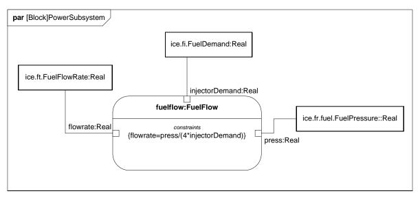
Figure B.24 - Defining Fuel Flow Constraints (Parametric Diagram)
