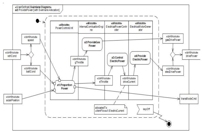
Figure B.35 - Detailed Behavior Model for "Provide Power" (Activity Diagram) Note hierarchical consistency with Figure B.33.
