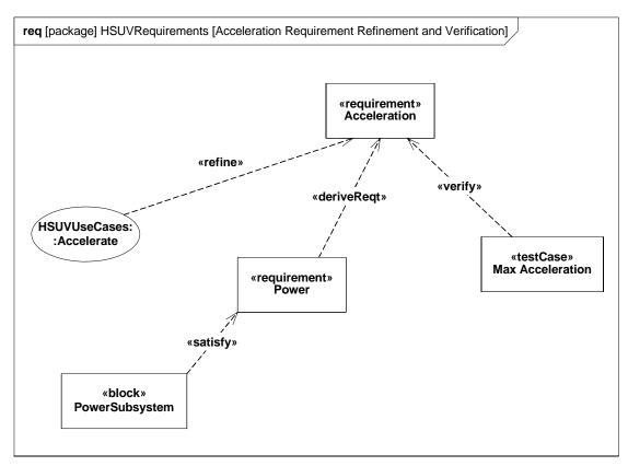
Figure B.13 - Acceleration Requirement Relationships (Requirements Diagram)
