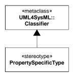
Figure 8.6 - Abstract syntax extensions for SysML property-specific types
