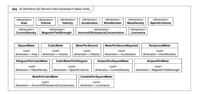
Figure C.6 - SI Derived Units Expressed In Base Units
