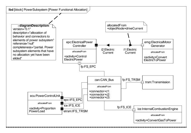
Figure 15.10 - Internal Block Diagram Showing Allocation for HybridSUV Accelerate Example
