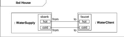
Figure 8.14 - Two views of Water Delivery connector within House block
