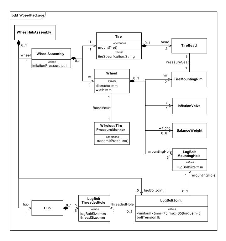
Figure 8.8 - Block diagram for the Wheel Package
