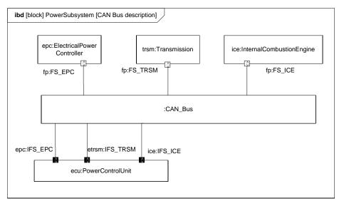
Figure B.22 - Consolidating Interfaces into the CAN Bus. (Internal Block Diagram)
