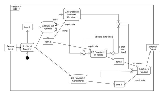
Figure C.1 - Example activity with «effbd» stereotype applied
