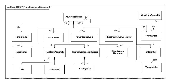
Figure B.18 - Defining Structure of Power Subsystem (Block Definition Diagram)
