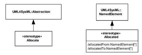
Figure 15.1 - Abstract syntax extensions for SysML Allocation
