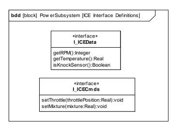
Figure 9.4 - Interfaces "ctrl" standard port of InternalCombustionEngine
