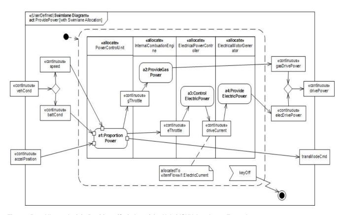
Figure 15.9 - AllocateActivityPartitions (Swimlanes) for HybridSUV Accelerate Example
