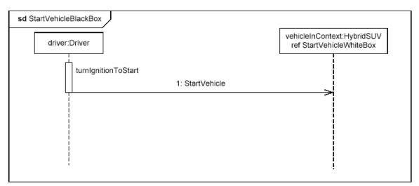
Figure B.9 - Black Box Interaction for "StartVehicle," referencing White Box Interaction (Sequence Diagram)
