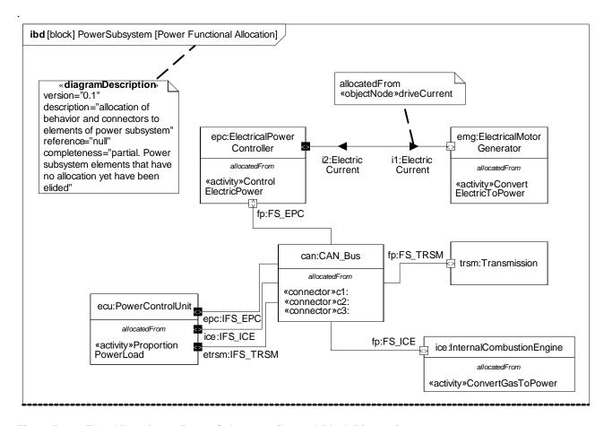
Figure B.36 - Flow Allocation to Power Subsystem (Internal Block Diagram)
