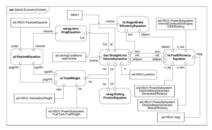
Figure B.29 - Establishing Mathematical Relationships for Fuel Economy Calculations (Parametric Diagram)
