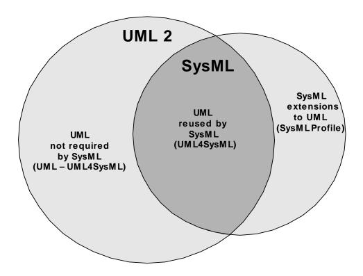
Figure 4.1 - Overview of SysML/UML interrelationship
