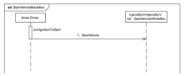
Figure 12.2 - Black box interaction during "starting the Hybrid SUV"
