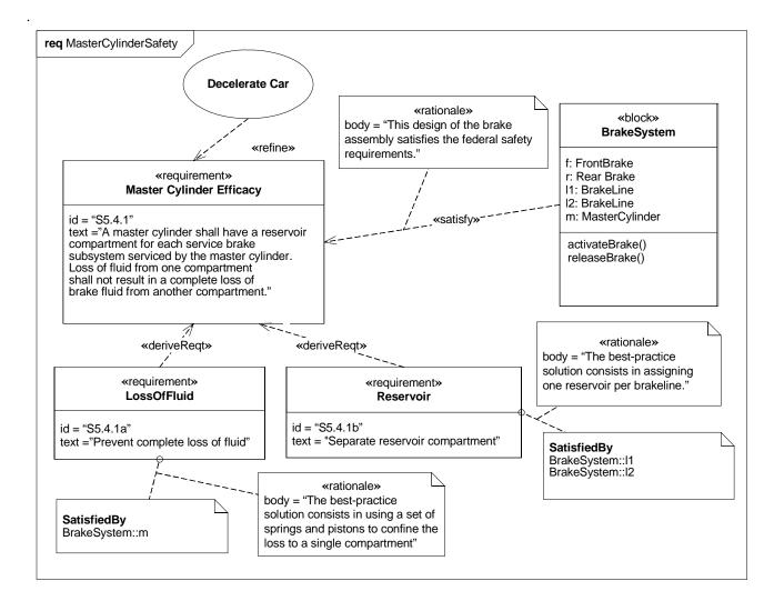
Figure 16.4 - Links between requirements and design
