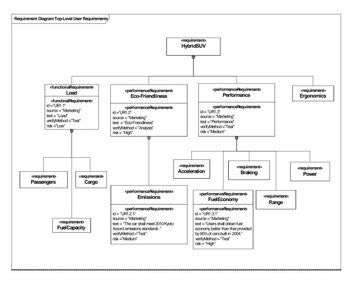
Figure C.3 - Example extensions to Requirement
