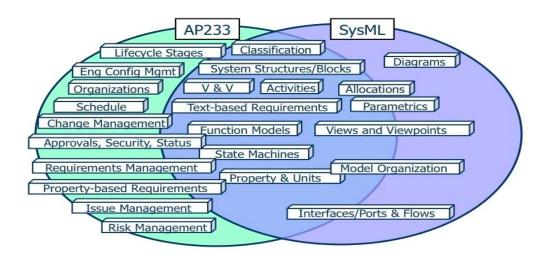
Figure D.1 - SysML/AP233 Data Overlaps
