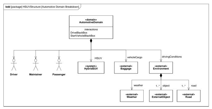
Figure B.15 - Defining the Automotive Domain (compare with Figure B.4) - (Block Definition Diagram)
