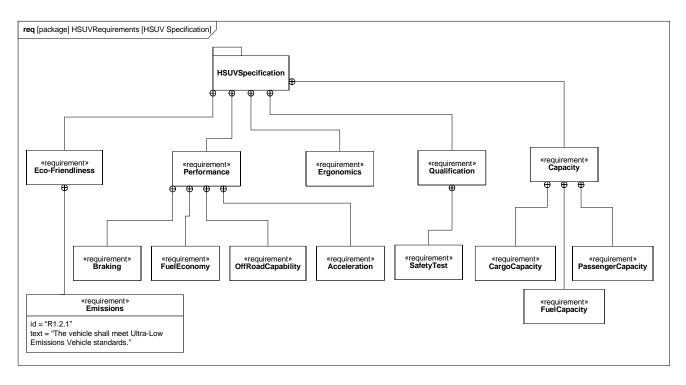
Figure B.11 - Establishing HSUV Requirements Hierarchy (containment) - (Requirements Diagram)
