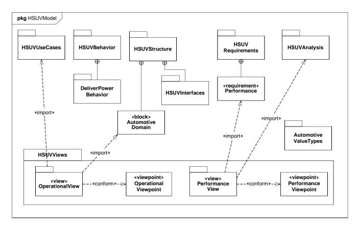
Figure B.3 - Establishing Structure of the User Model using Packages and Views (Package Diagram)
