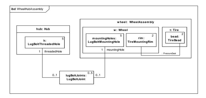
Figure 8.9 - Internal Block Diagram for WheelHubAssembly
