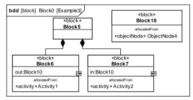
Figure 15.7 - Example of flow allocation from ObjectNode to FlowProperty
