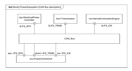
Figure B.22 - Consolidating Interfaces into the CAN Bus. (Internal Block Diagram)
