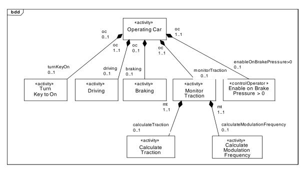
Figure 11.13 - Example block definition diagram for activity decomposition
