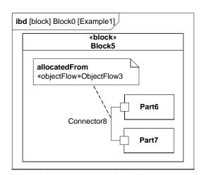
Figure 15.5 - Example of flow allocation from ObjectFlow to Connector
