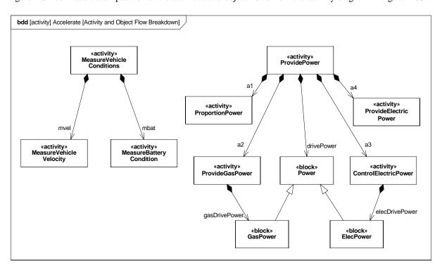
Figure B.34 - Decomposition of "Accelerate" Function (Block Definition diagram)
