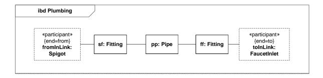
Figure 8.16 - Internal structure of Plumbing association block
