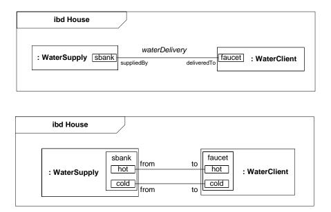
Figure 8.13 - Two views of Water Delivery connector within House block
