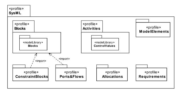
Figure 4.3 - SysML Package Structure
