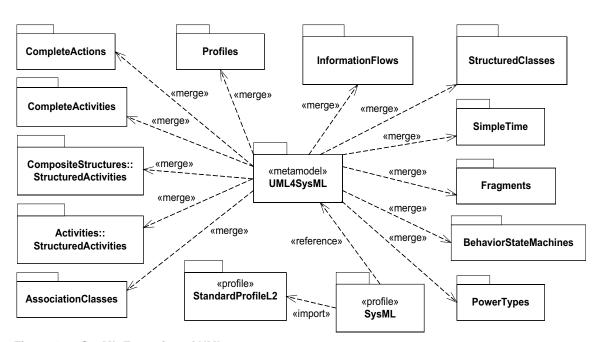
Figure 4.2 - SysML Extension of UML
