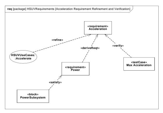
Figure B.13 - Acceleration Requirement Relationships (Requirements Diagram)
