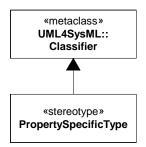
Figure 8.6 - Abstract syntax extensions for SysML property-specific types
