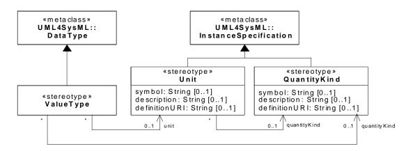
Figure 8.4 - Abstract syntax extensions for SysML value types
