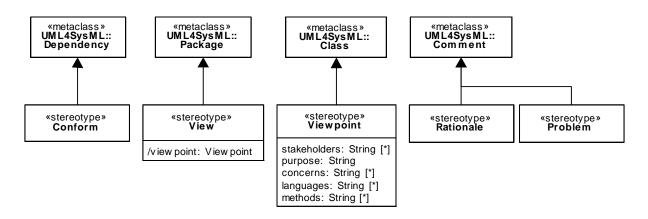
Figure 7.1 - Stereotypes defined in package ModelElements
