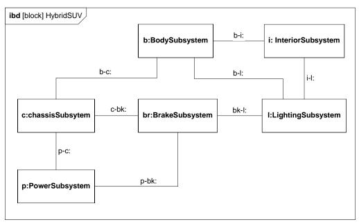
Figure B.17 - Internal Structure of Hybrid SUV (Internal Block Diagram)
