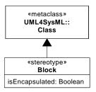
Figure 8.2 - Stereotypes defined in SysML Blocks package
