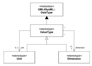
Figure 8.4 - Abstract syntax extensions for SysML value types
