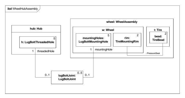
Figure 8.8 - Internal Block Diagram for WheelHubAssembly
