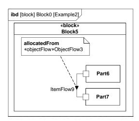
Figure 15.6 - Example of flow allocation from ObjectFlow to ItemFlow
