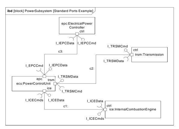
Figure 9.3 - Usage Example of StandardPorts
