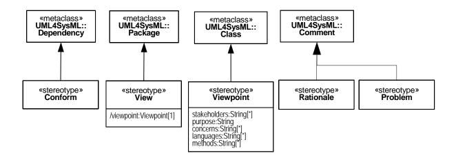
Figure 7.2 - Stereotypes defined in package ModelElements.
