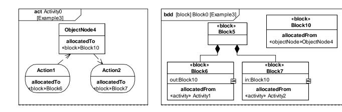
Figure 15.7 - Example of flow allocation from ObjectNode to FlowProperty
