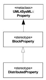
Figure 8.3 - Abstract syntax extensions for SysML properties
