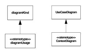
Figure A.3 - Diagram Usages
