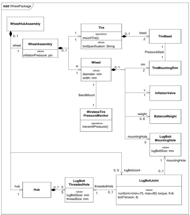
Figure 8.7 - Block diagram for the Wheel Package
