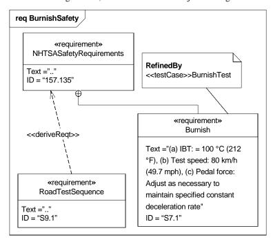
Figure 16.7 - Linkage of a Test Case to a requirement: This figure shows the Requirement Diagram.
