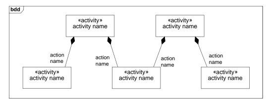
Figure 11.1 - Block definition diagram with activities as blocks.
