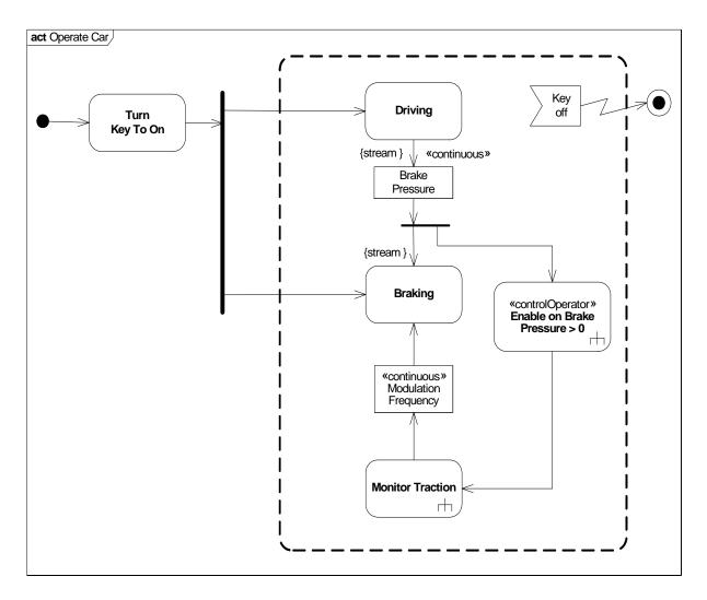
Figure 11.10 - Continuous system example 1.
