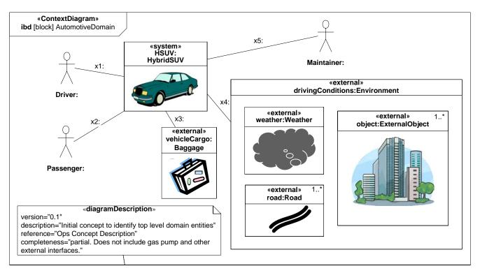
Figure B.4 - Establishing the Context of the Hybrid SUV System using a User-Defined Context Diagram. (Internal Block Diagram) Completeness of Diagram Noted in Diagram Description
