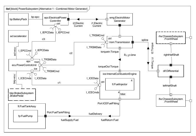
Figure B.19 - Internal Structure of the Power Sybsystem (Internal Block Diagram)
