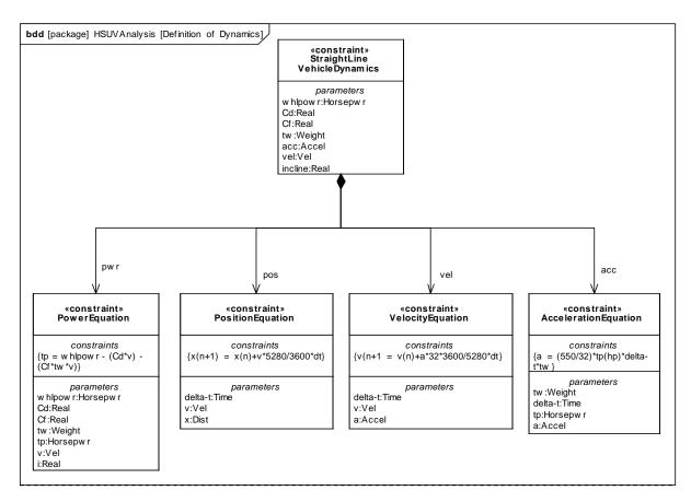
Figure 10.2 - Constraint block definitions in a Block Definition diagram
