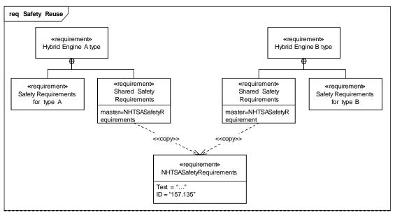
Figure 16.6 - Use of the copy dependency to facilitate reuse
