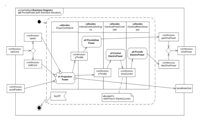
Figure B.35 - Detailed Behavior Model for "Provide Power" (Activity Diagram) Note hierarchical consistency with Figure B.33.
